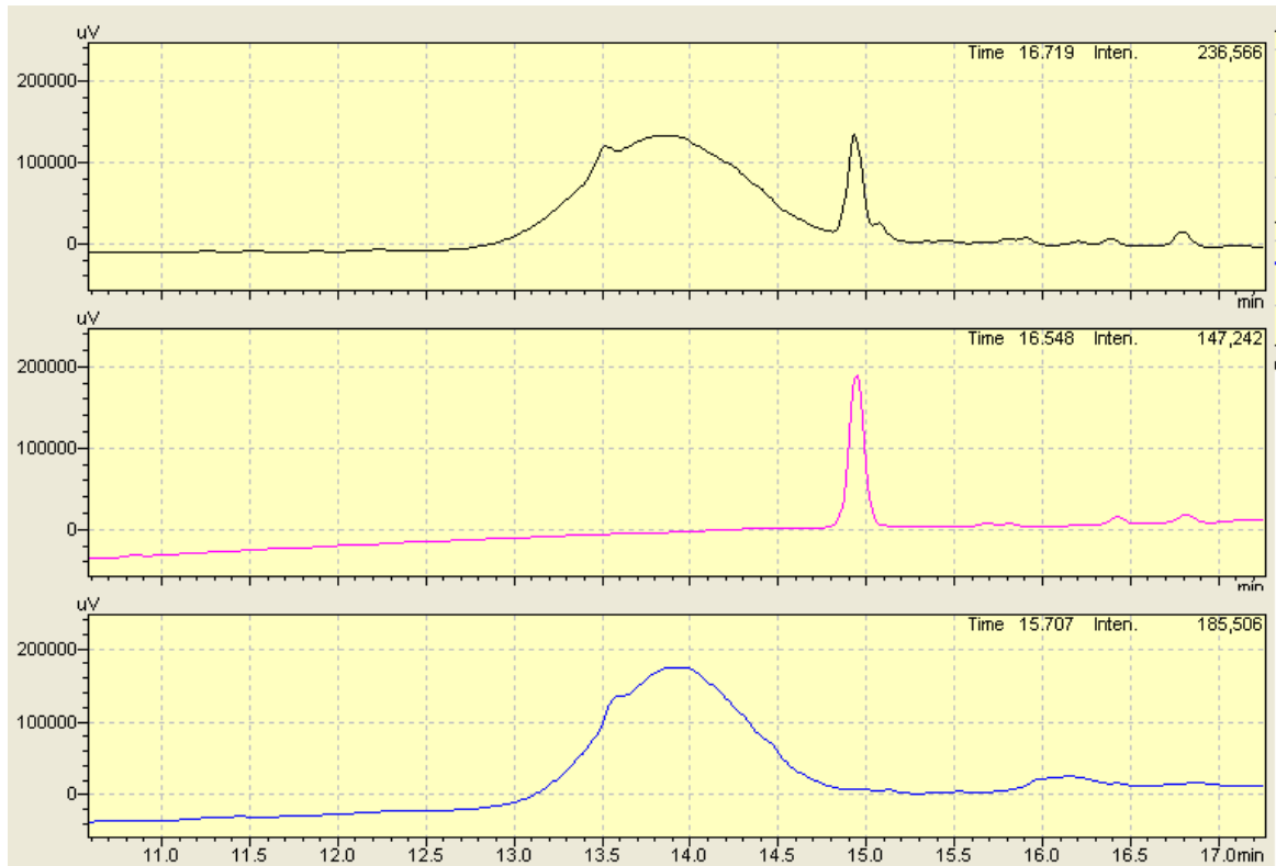
Figure 3.3 Representative chromatogram of (A) MDL-28170-encapsulated PCADK particles (B) MDL-28170 standard solution, and (C) blank PCADK microparticles from reverse phase HPLC.
